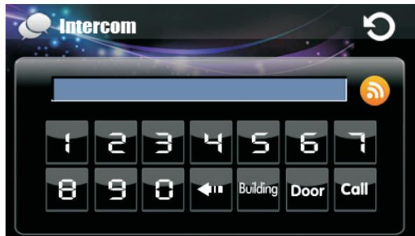
Input 4 digits of Building No. +2 digits of Door No. + 4 digits of Room No., then press icon to call the resident. For example, if input Building 0001, Door 01, Room 0001, you can input "1" + "Building" + 1 + "Door" +1, the system will add zero automatically. If input wrong, click to delete. If the Building No. and Door No. is consistent, you can also input Room No. directly.
